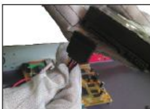
2.Connect hard disk data line.
