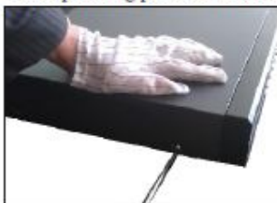
6.Fix the screws of the top cover .
