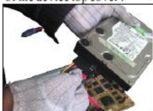
3.Connect hard disk power line
